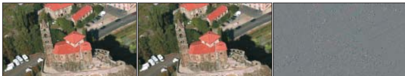
Left: Original image Center: Intra-frame predictive image Right: Difference image obtained from subtracting the intra-frame predictive image from the original image. This shows the high accuracy of intra prediction.
